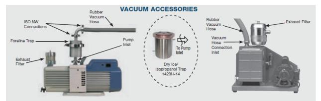
Exhaust Filter - Connects to pump's outlet. Filters oil mist from the pump's exhaust to keep your working area clean and air quality healthful. A second option is an exhaust line to a vapor hood or other outside exhaust vent. This requires an adapter and air tight connections (see p. 40).
